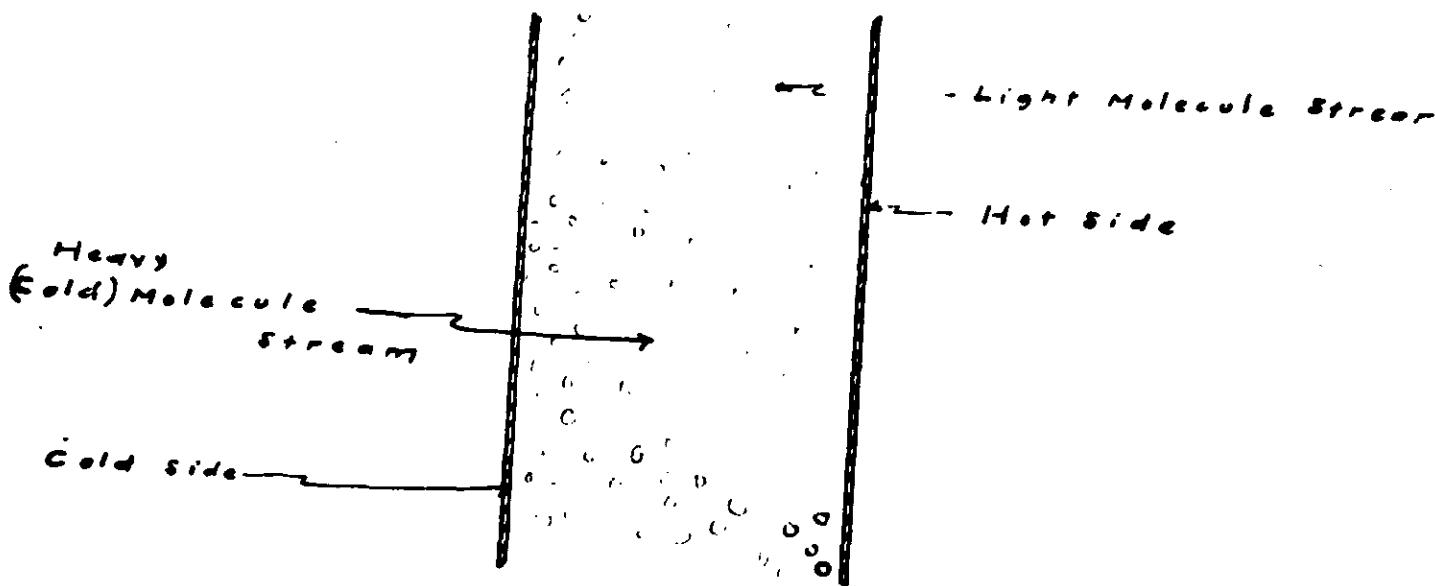
As is shown, in most cases the lighter molecules will concentrate toward the top of the apparatus.
